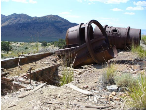
Bruckner's roasting cylinders at the Tenabo Mill.
