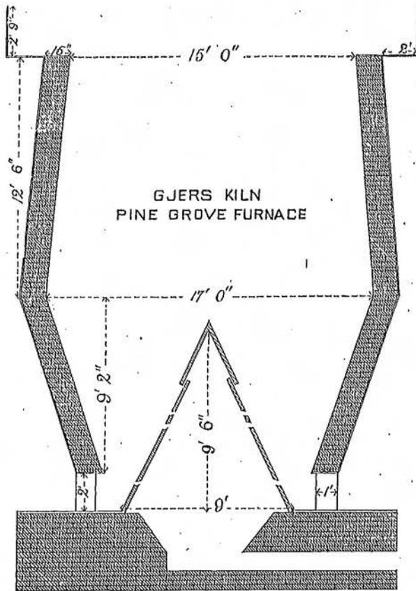
Figure 1. Gjers Kiln, Pine Grove Furnace (Ohio) reveals the masonry construction and the gravity-aided design whereby molten metal flows to the base of the furnace. (from N. W. Lord, "Iron Manufacture of Ohio" in *Economic Geology*, 1884)
