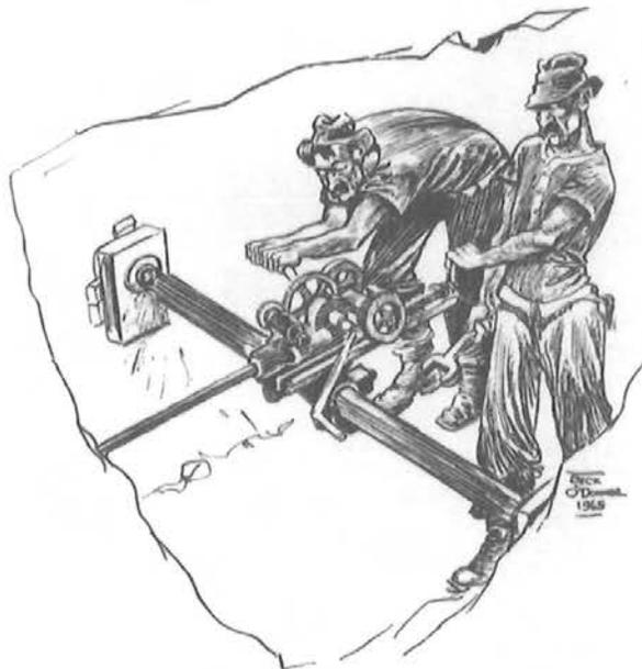
*The Hand Crank Rock Drill. The crank compresses a spring that, when released, strikes the drill rod penetrating the rock. (Buck O'Donnell, Yesterday's Mining, 1966. Courtesy of Gene Skinner.)*
