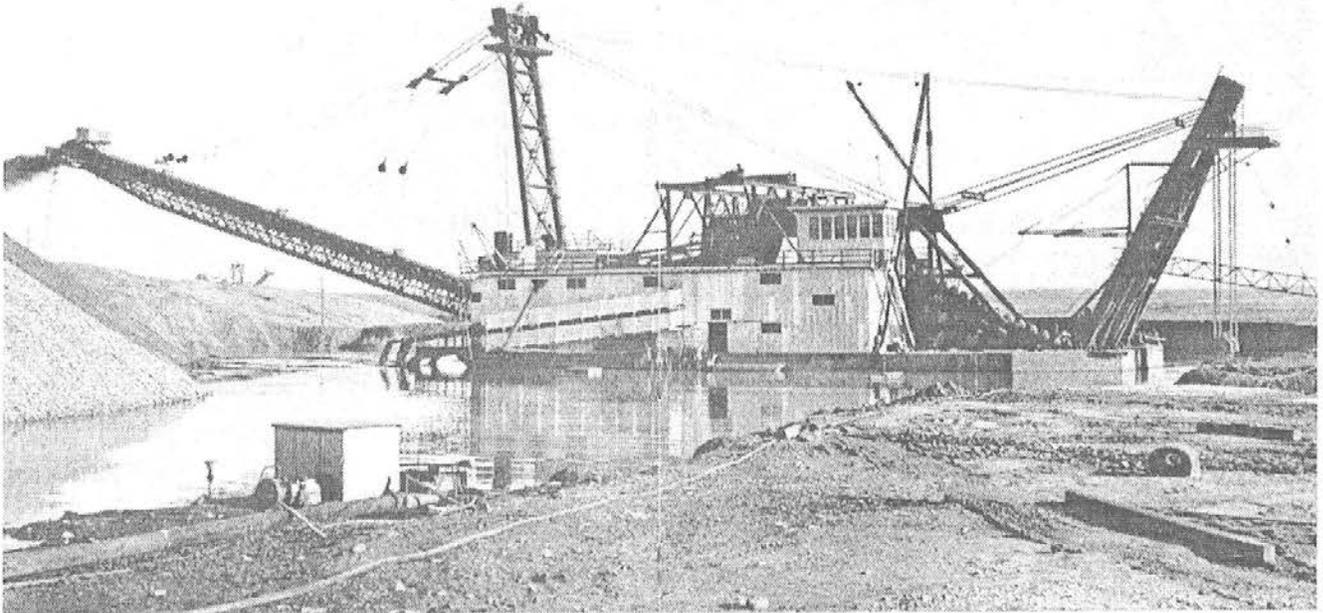
Figure 10 Capital Dredging Co., Dredge #4. Built by Yuba, 1937. Equipped with 18 cubic foot buckets which dug to 82 feet below water level. From *Yuba Placer Mining Dredges*, 1952.
