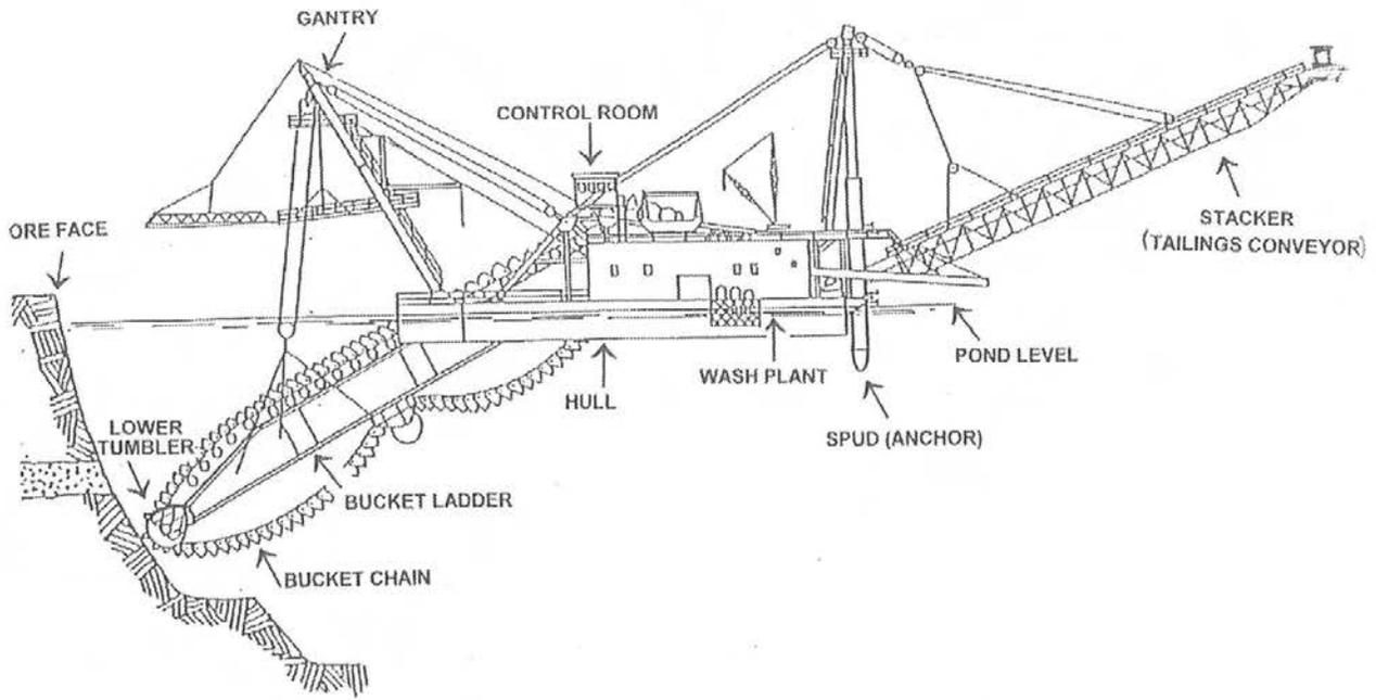
Figure 1 Schematic diagram of floating bucket-line dredge. From files of N. W. Kirshenbaum.
